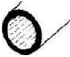
EXIT PORT OF FIRAS ANTENNA DIA: 3.98 cm FREQ. RANGE: 10 – 600 GHz (a)
